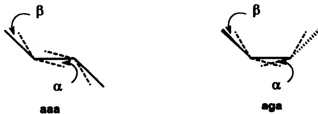
Figure 4. Schematic representations of C-O and C-C bond paths and O-C-C path angles for the aaa and aga conformers of 1,2-dimethoxyethane (DME) as derived from 3-21G, 6-31G* and 6-311+G(3df) wavefunctions. The values of \alpha and \beta and the difference between path angles and geometry angles (Table 5), uniquely define the direction in which C-O and C-C bond paths deviate from their corresponding axes.
